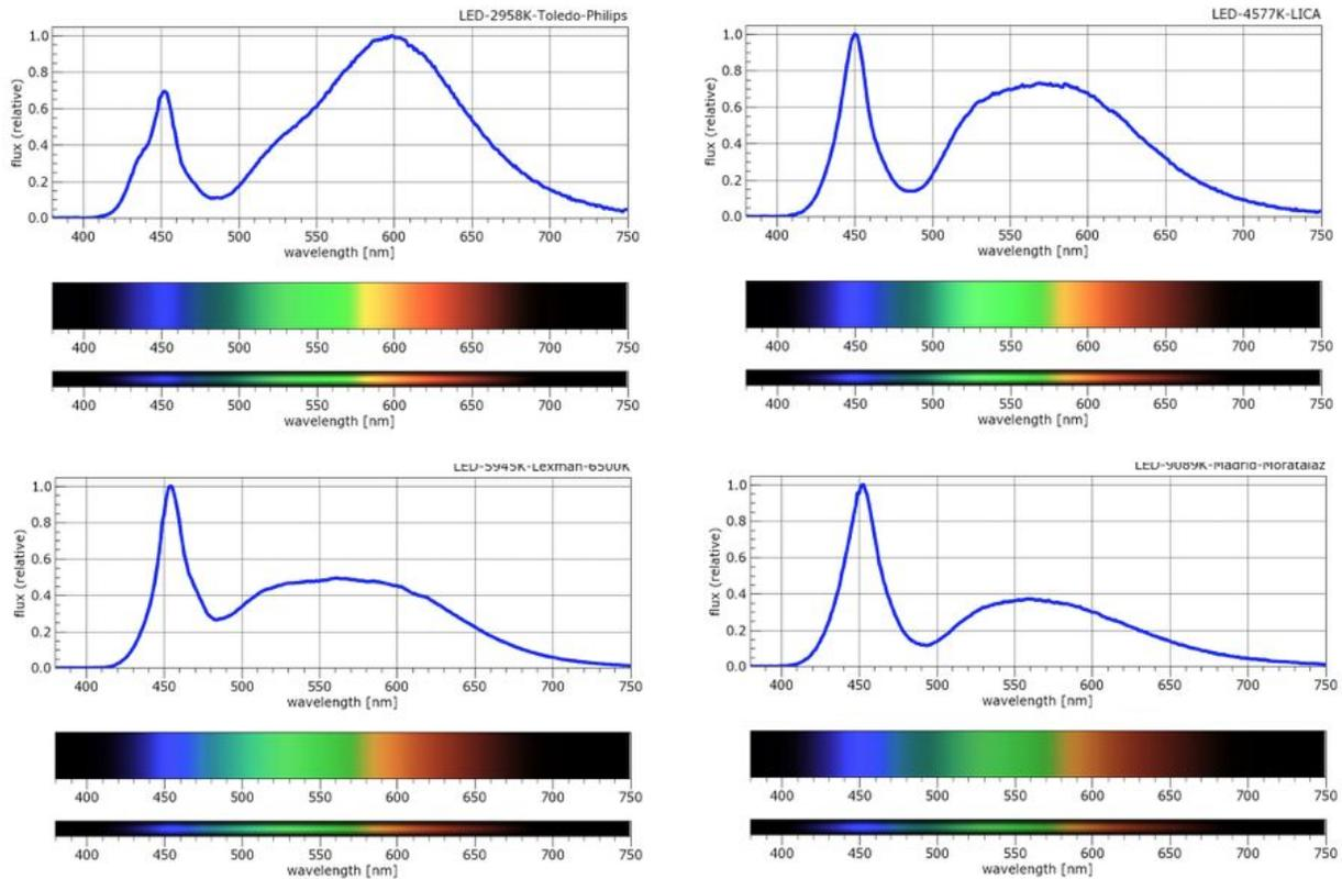
Figure 25a. Example of LED lamps of different colors.
