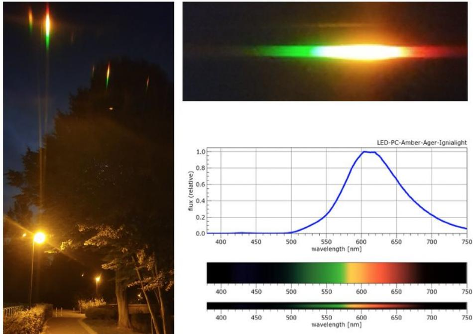
Figure 25b. PC amber LED lamp. Picture taken at Rheda-Wiedenbrück (Germany) by Andreas Hänel (left). The color of the lamp is orange and the spectrum does not show any blue light (upper right).
