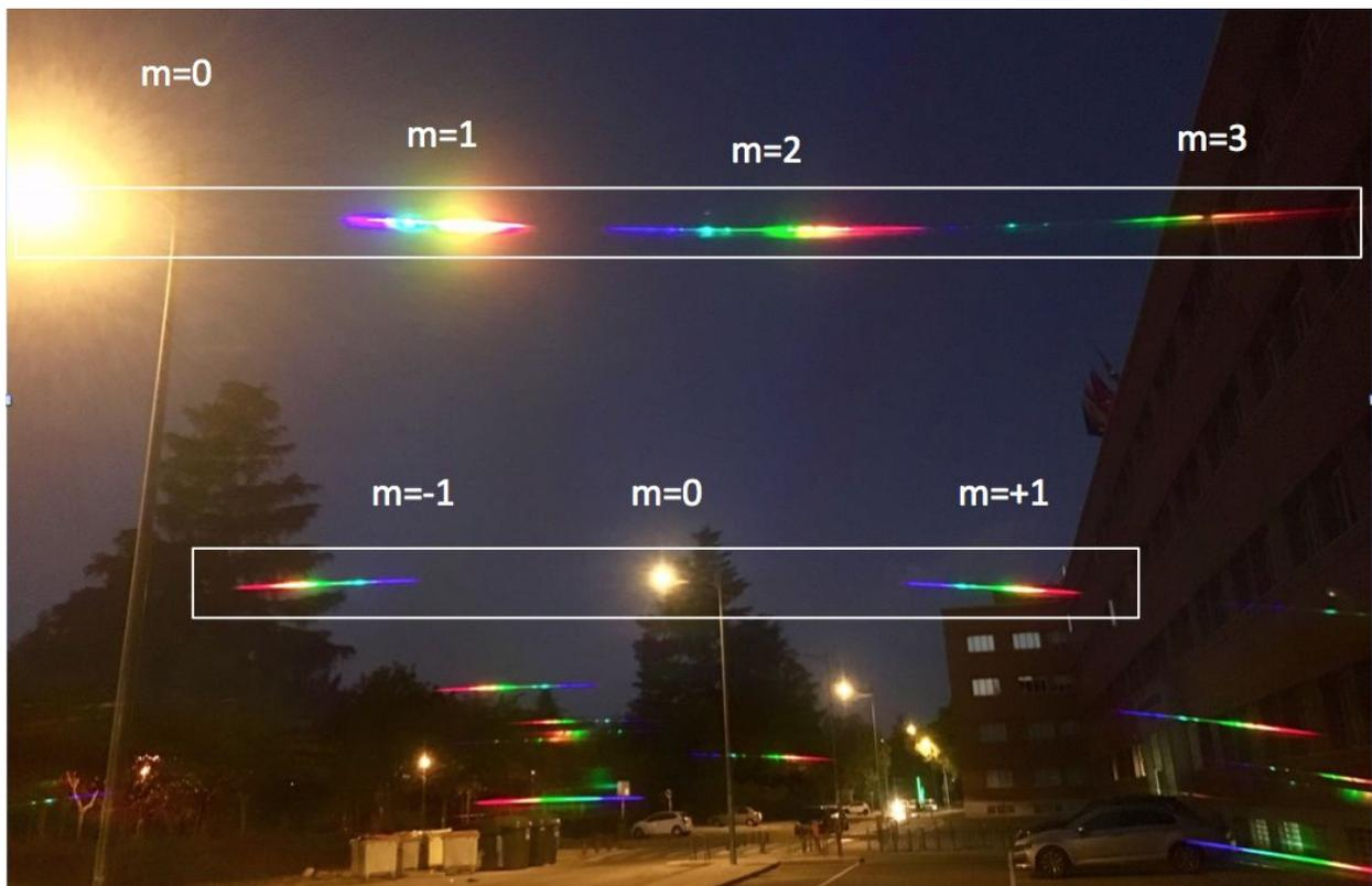
Figure 7. Annotated grating orders for two light sources. See text for explanation.
