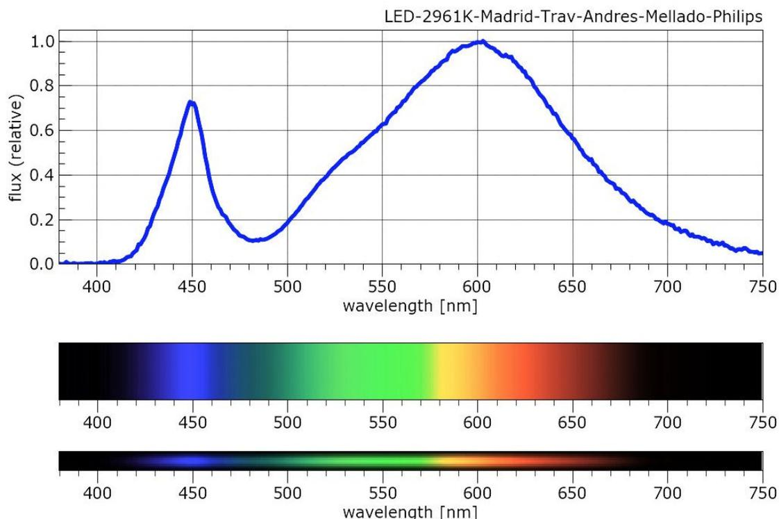
Figure 24. Example of LED lamp spectrum from the LICA-UCM lamp spectra database.
