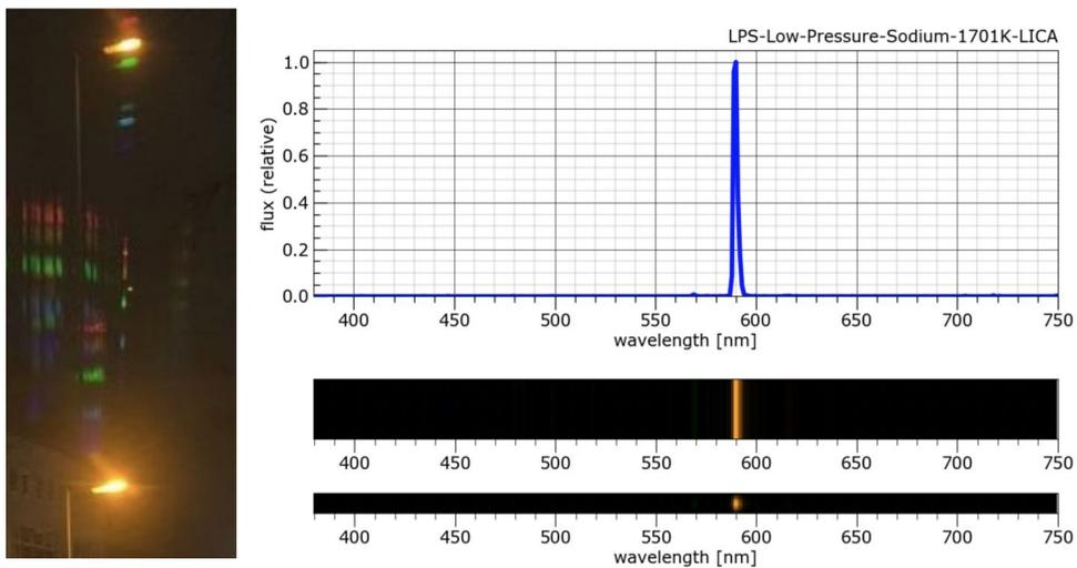
Figure 25c. LPS lamp and its spectrum (left). Picture taken at Erasmus University Rotterdam campus. Only the sodium orange line is prominent.
