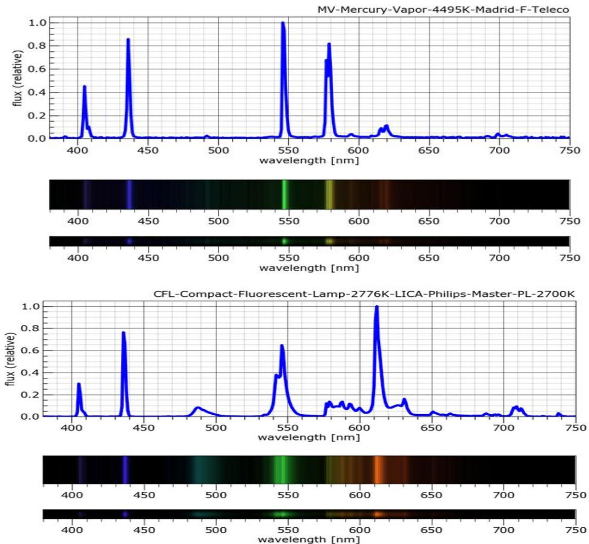
Figure 27. Two of the spectra of the LICA-UCM lamps spectral database showing the plots and a visual rendering of the color spectra.
