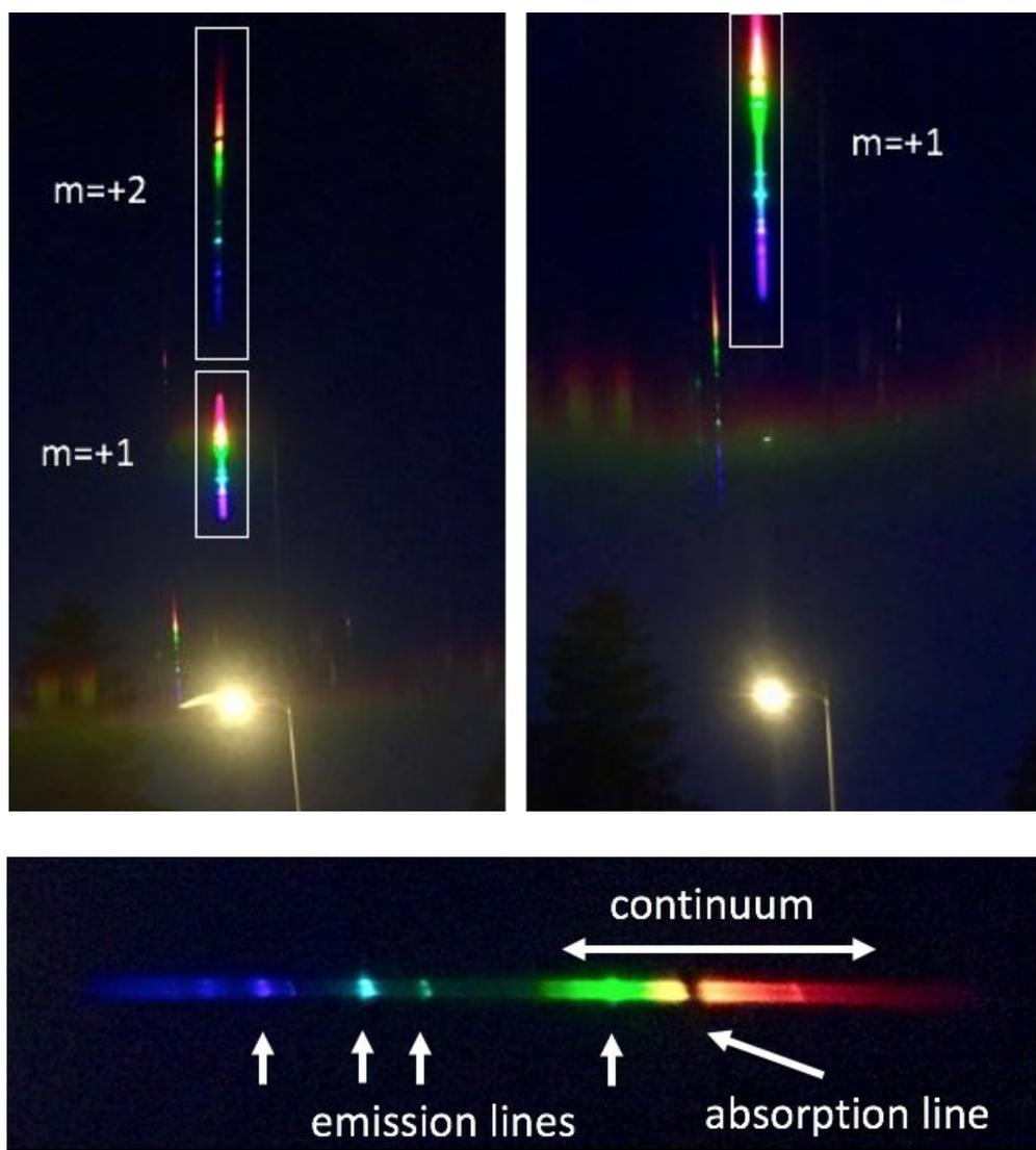
Figure 8. Same HPS lamp pictured with a 500 lines/mm grating (left) and 1000 lines/mm grating (right) showing the differences in linear dispersion. Principal features of a spectrum (bottom).
