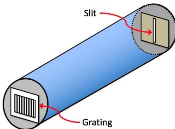
Figure 31. Visual spectroscope sketch.
