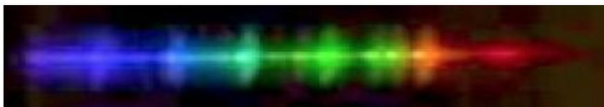
Figure 23. Spectrum of street MH lamp.
