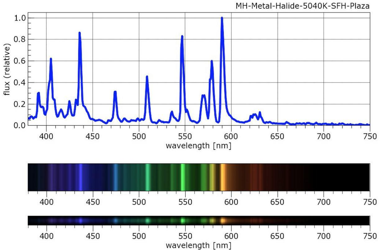
Figure 22. Example of MH lamp spectrum from the LICA-UCM lamp spectra database. Besides the emission lines of MV lamps they are some additional lines as the yellow 591 nm line.
