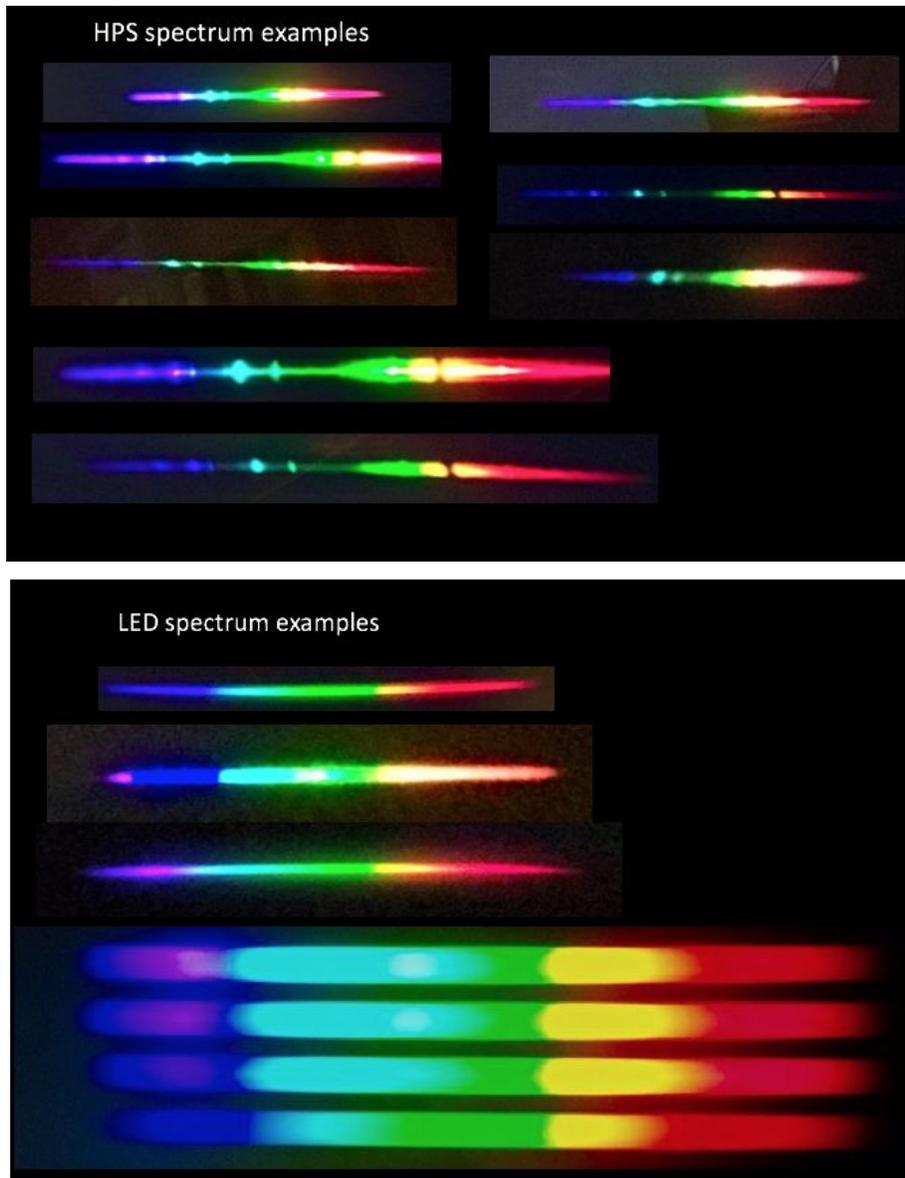
Figure 28. Examples of spectra taken with smartphone and grating for HPS and LED lamps.
