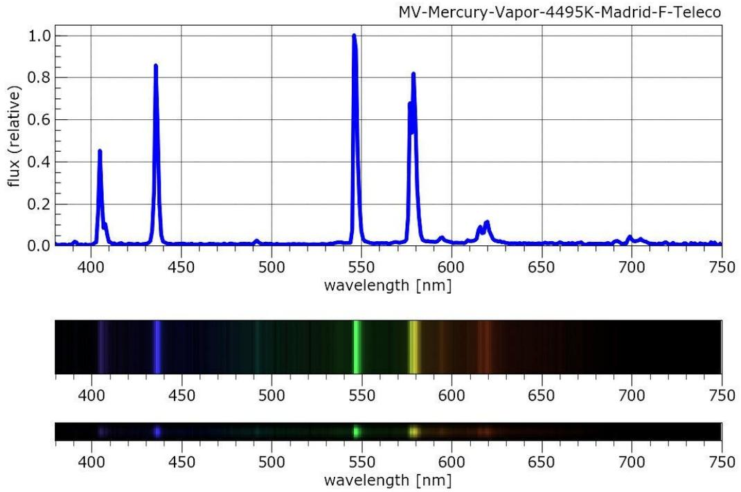
Figure 20. Example of MV lamp spectrum from the LICA-UCM lamp spectra database.
