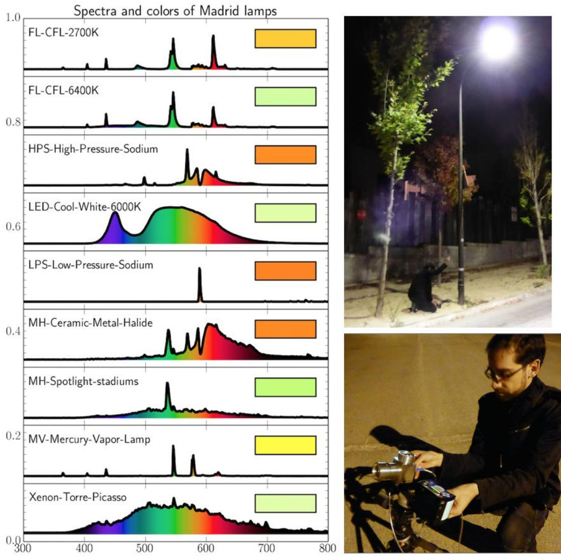
Figure 3. A collection of typical spectra of lamps collected in Madrid urban area and the researcher using a portable spectrograph to obtain the data in situ.
