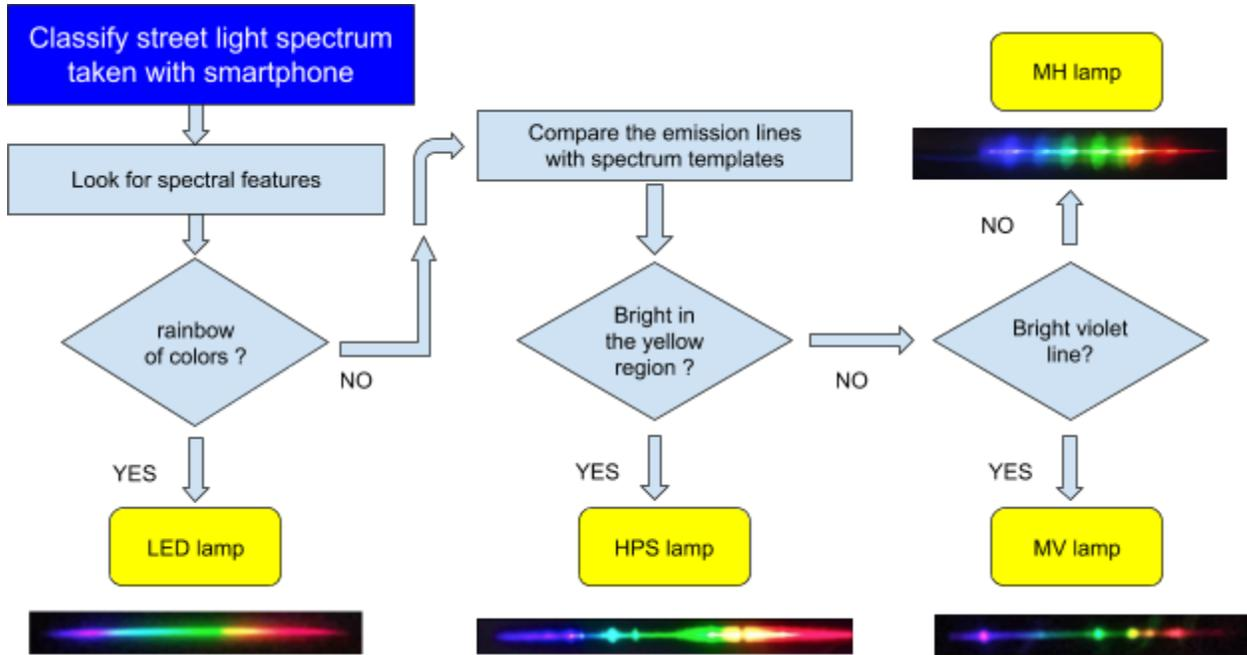
Figure 26. Flowchart to help on lamp classification according to the spectrum.
