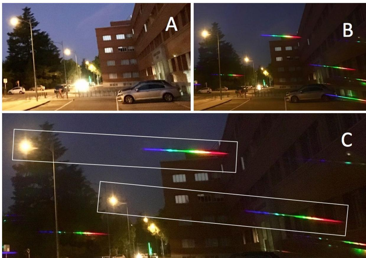
Figure 6. Spectra of HPS lamps obtained with a transmission grating and recorded with a smartphone. (A) Direct picture obtained with the phone. (B) Picture taken at the same place after placing a grating over the camera lens. (C) Detail of two of the lamps with their corresponding spectrum.
