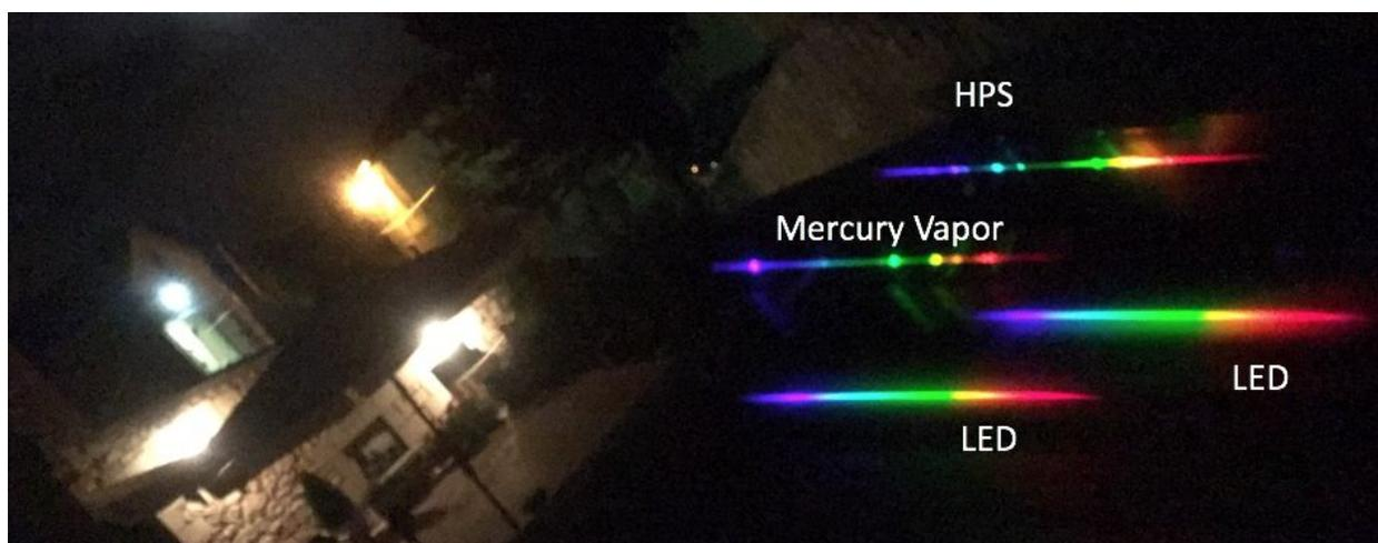
Figure 2. Picture of lamps and their spectra taken at night in a location with mixed illumination luminaries.
