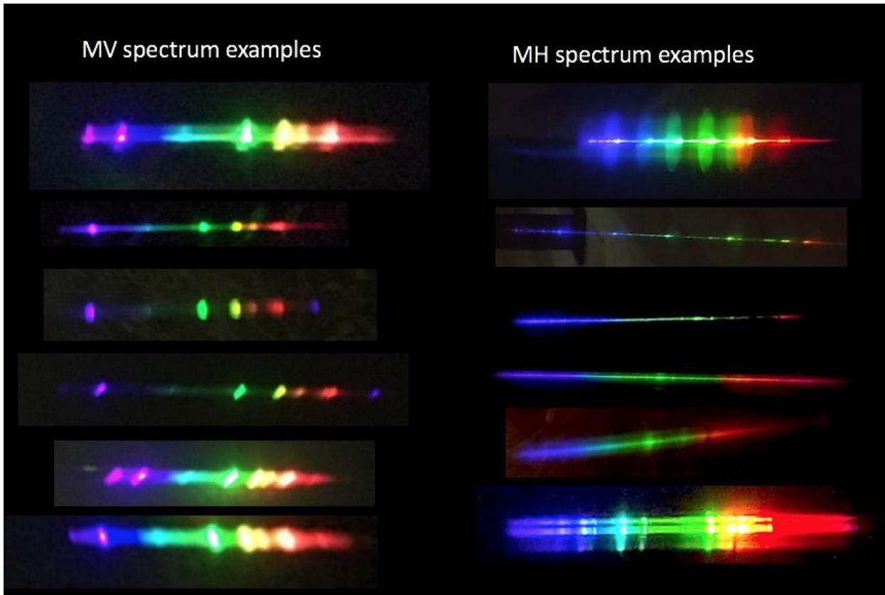
Figure 29. Examples of spectra taken with smartphone and grating for MV and MH lamps.
