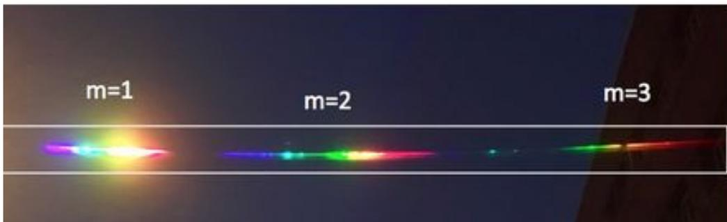
Figure 19. Spectrum of street HPS. Order  $m=1$  is saturated but we can see in order  $m=2$  that most of the light is in the yellow part and some emission lines are present in the blue-green. In order  $m=3$  the absorption (dark lane) in the 589 nm splitting the yellow spectrum in two.
