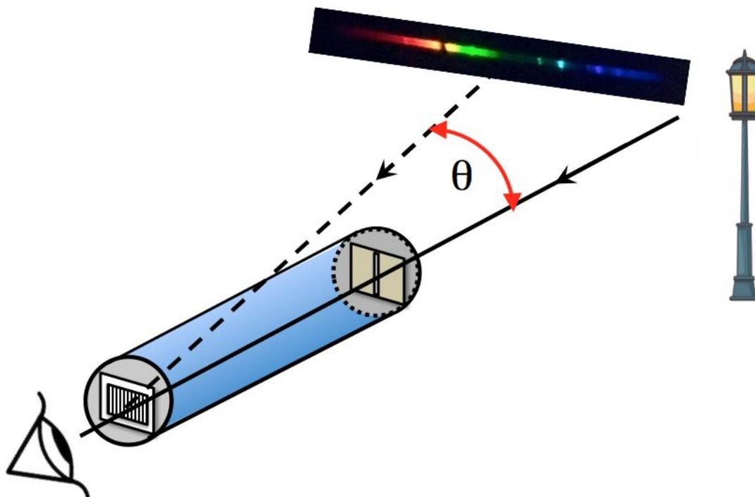
Figure 32. Using the visual spectroscope.
