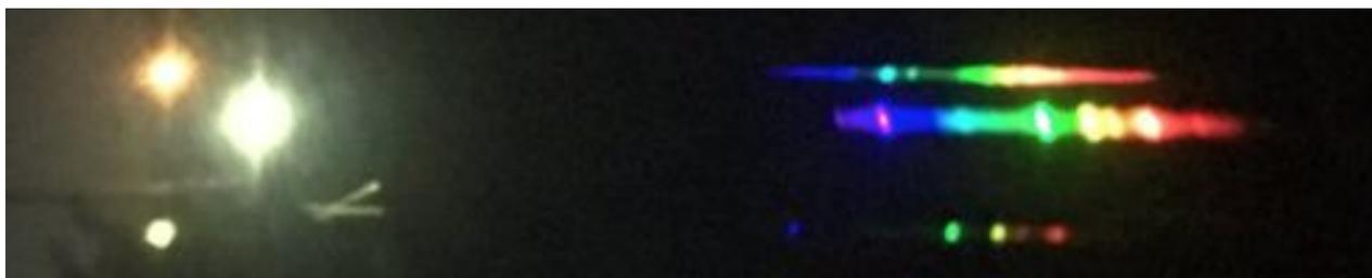
Figure 17. Three different lamps in the same location allows us to compare their spectra obtained at the same time with a single picture. From top to bottom: HPS, MH, and MV lamps.
