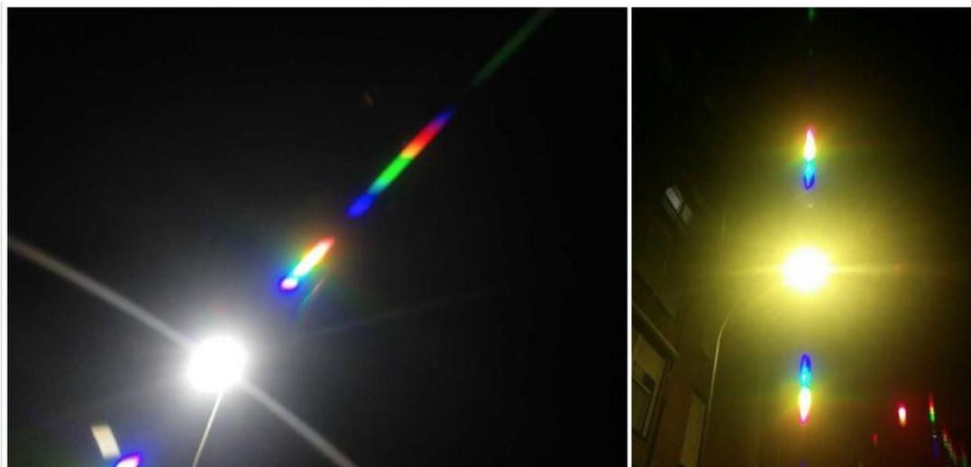
Figure 10. Spectra of sources taken too close to the lamps showing saturated spectra.
