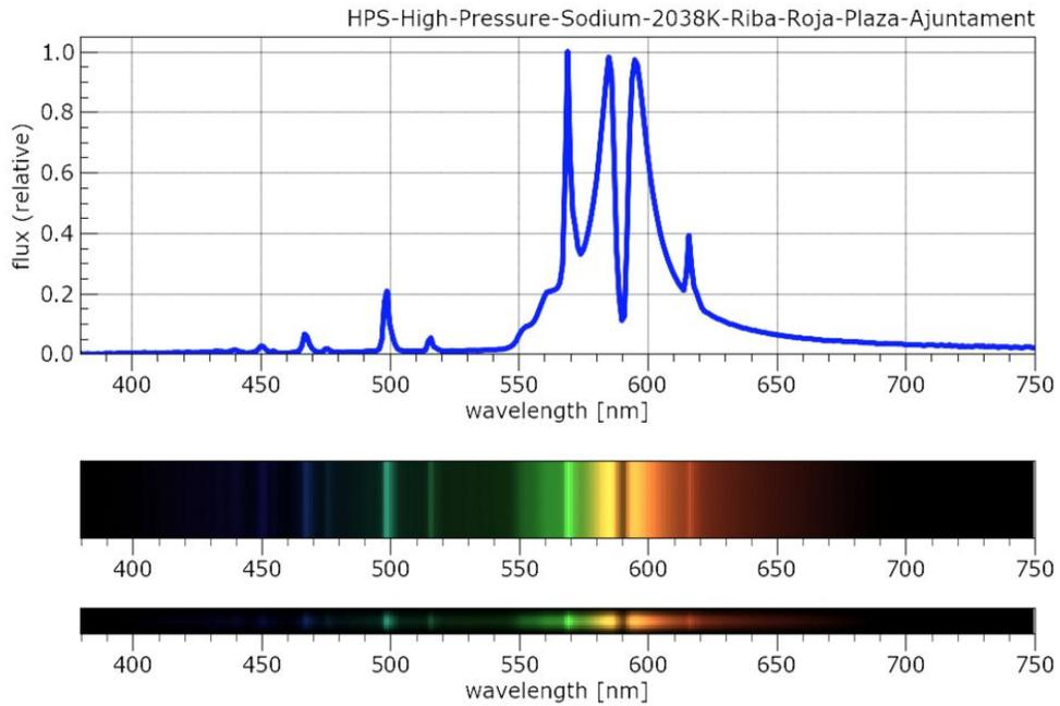
Figure 18. Example of Sodium HPS lamp from the LICA-UCM lamp spectra database.
