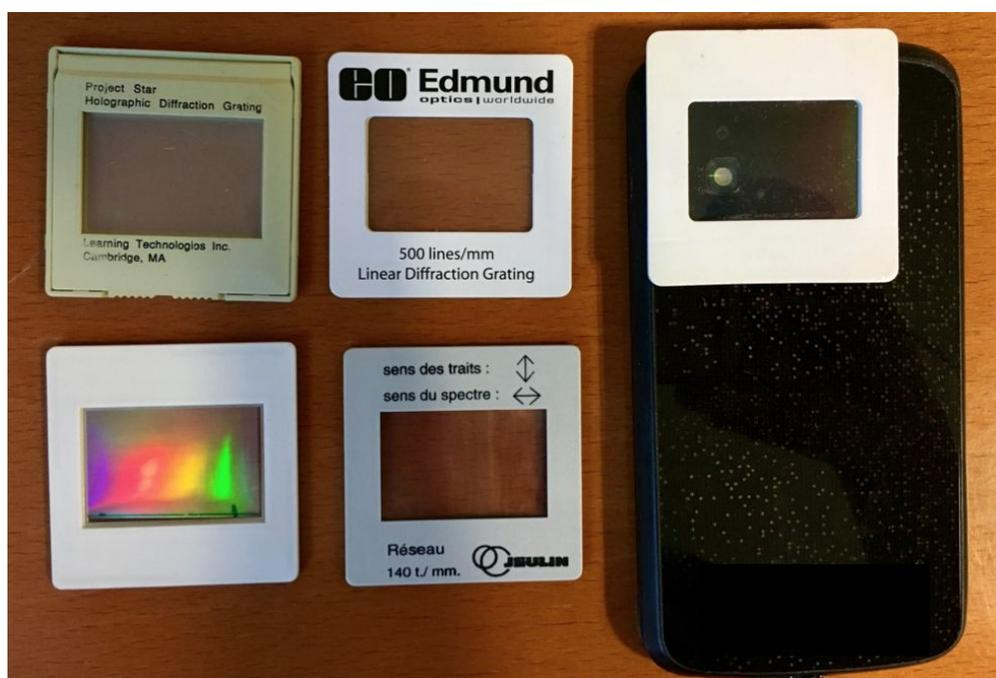
Figure 5a. Smartphone with a transmission grating covering the lens of the camera and some examples of transmission gratings.
