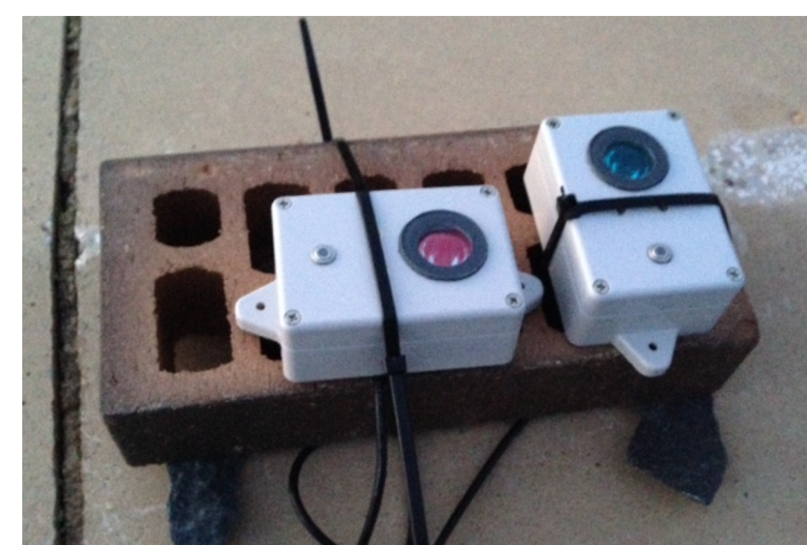
Figure 1. TESS photometer prototypes (with dichroic and color filters) being tested under dark skies during the LoNNe intercomparison campaign at Montsec.
